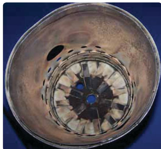
Figure 5-2. Inside view of a combustion chamber liner.
