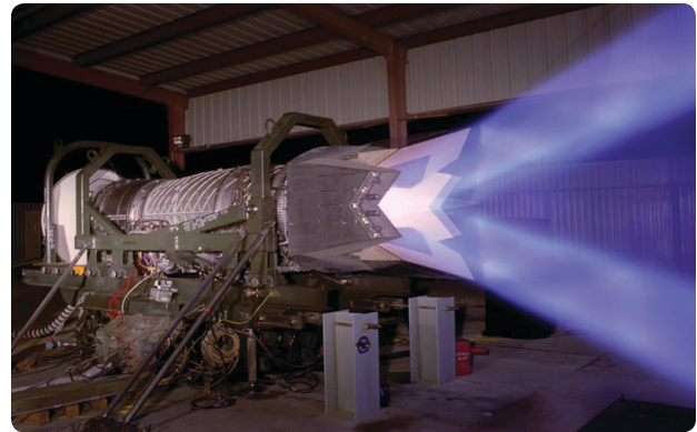
Figure 7-10. A pilot can direct thrust via the vectoring nozzle 20^\circ up or down to increase flight maneuverability.
