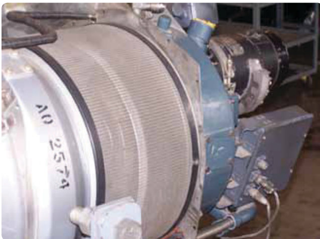
Figure 3-6. Example of a turboprop engine that incorporates inlet screens.
