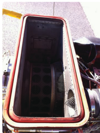
Figure 18-1. APU intake note FOD/ice screen around impeller.
