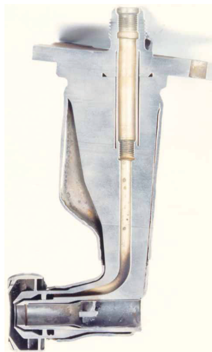
Figure 11-16. Simplex airblast nozzle cutaway.
