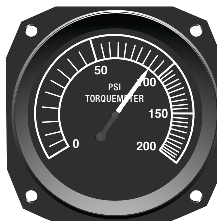
Figure 14-5. A typical analog torquemeter.
