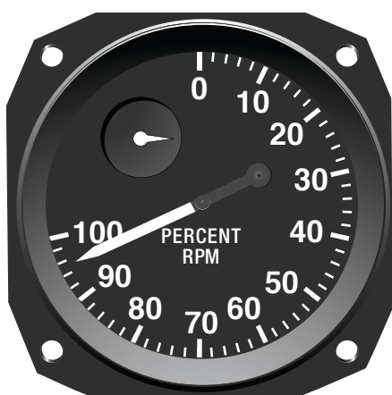
Figure 14-6. A typical analog RPM gauge.
