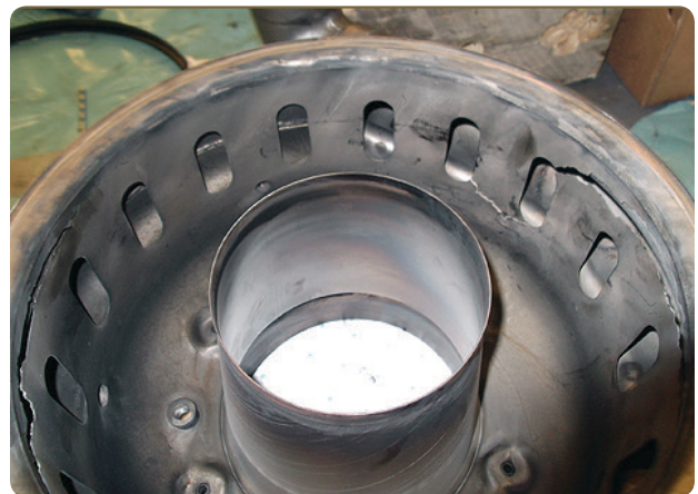
Figure 18-10. A typical APU hot section partially disassembled.
