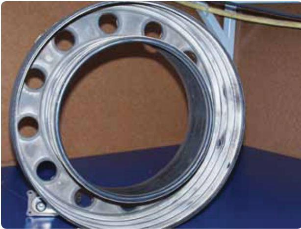
Figure 5-7. Annular combustion with chamber ceramic coating.
